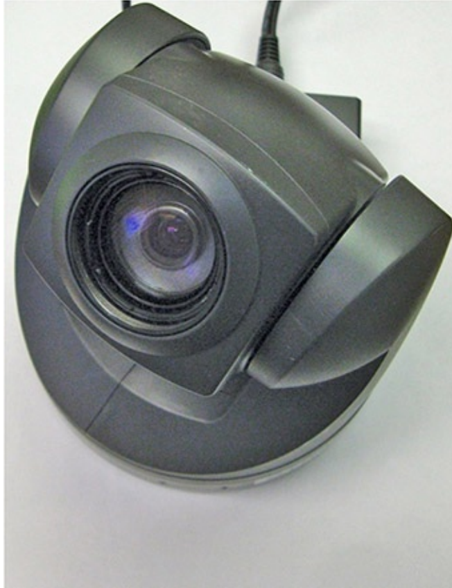
Figure 15-1 IP-based cameras leverage existing IP networks instead of needing a proprietary CCTV cable.
